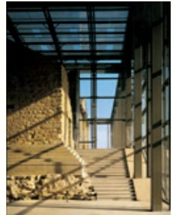
At Bougon, the lowest levels of the museum were built underground in the **chalky soil**. The museum's entrance, therefore, is around four metres below ground level at the bottom of the archaeological excavations. The chalky nature of the soil is underlined by the use of limestone paving slabs of different sizes and finishes.
